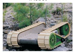
all terrain, including stairs 3 mt fall radio steering camera
