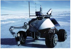
mobile camera spectrometer magnetometer compass mineral sampling
