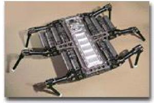
underwater, crab-like motion double-sided can be fitted with sensors
